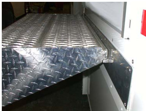
Figure 17: Stair Assembly (standard)
