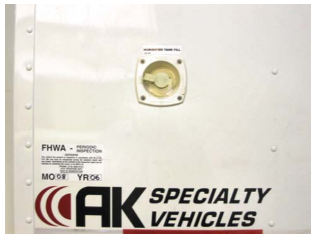
Figure 41: Humidifier External Water Connection
