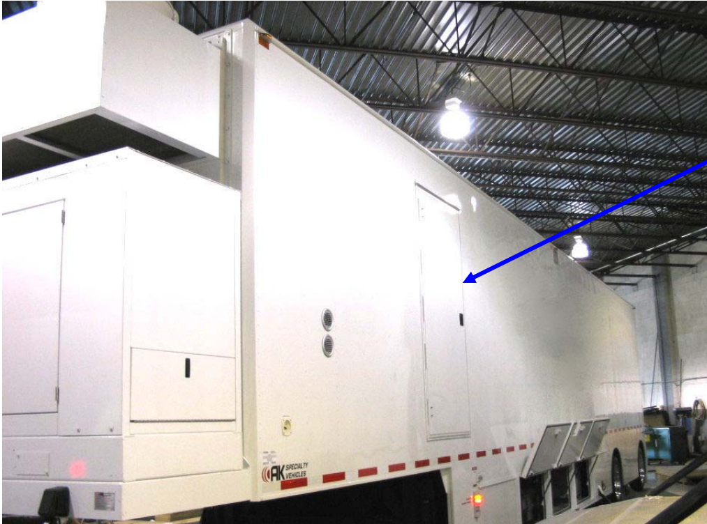
Figure 20: Emergency Exit / Service Door
