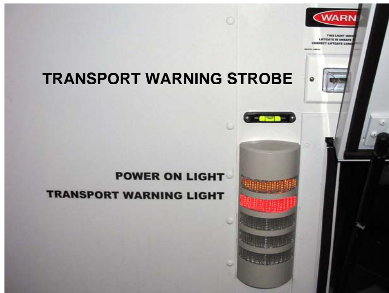
Figure 57: Lift Transport Warning Strobe
