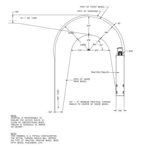
**Figure 7: Turning Requirements**
