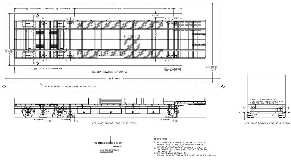
Figure 8: Tie Down Assembly (optional)
