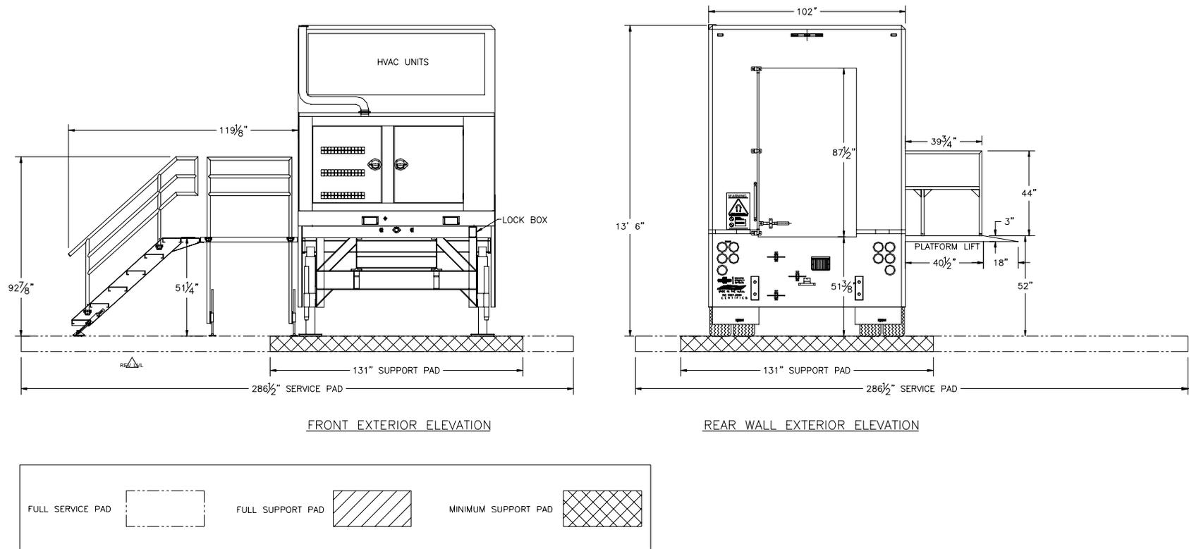
**Figure 5: Stair/Lift/Wall Elevation**
